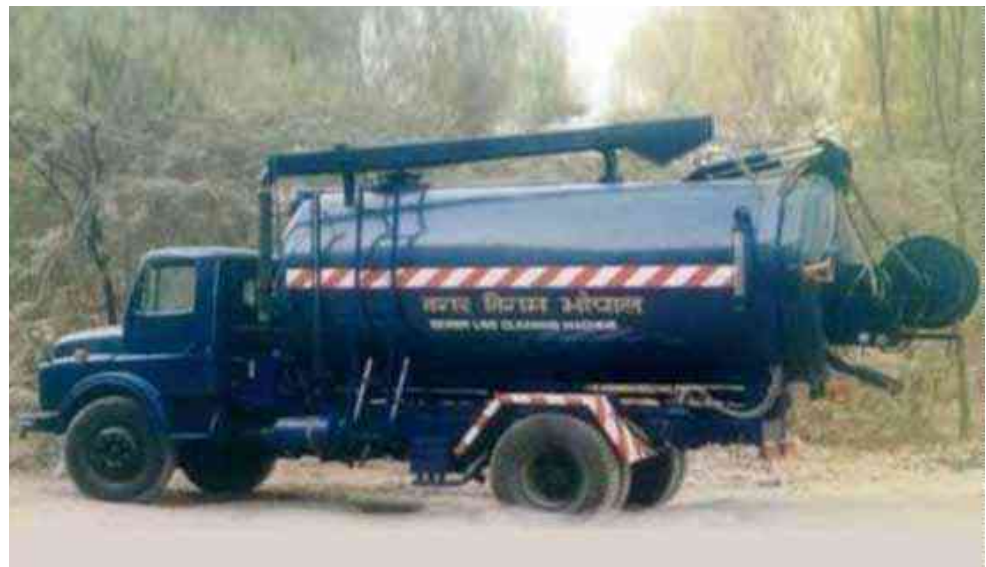
Figure 2.21: Truck Mounted with Pressure Water Jetting and Suction Machine 29
