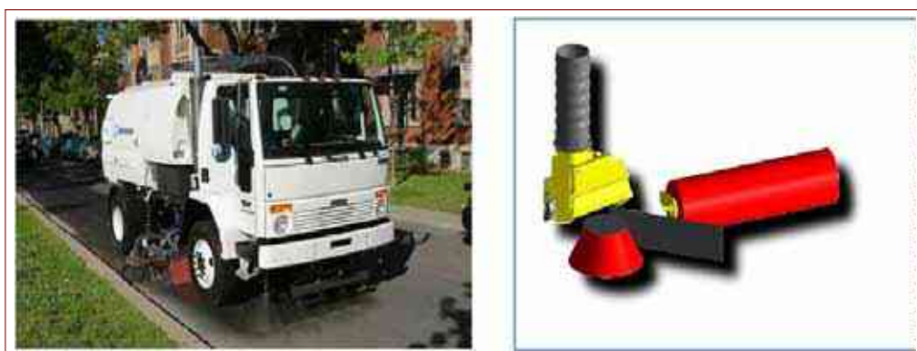
Figure 2.19: Vacuum Sweeper and Vacuum Nozzle 27
