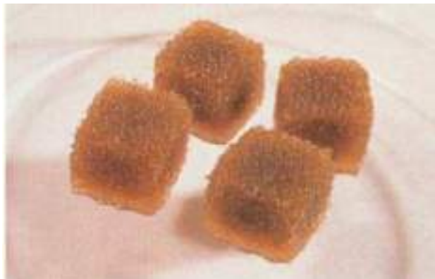
Figure 5.83 Linpor® Cubes carrying sludge (12x12x15 mm)
