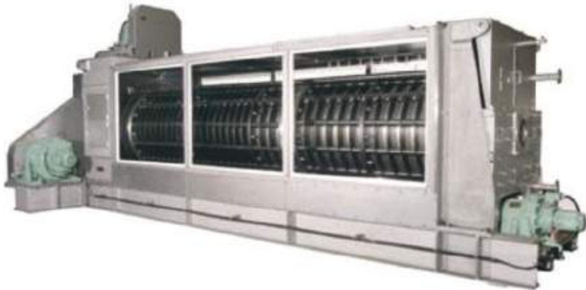
Figure 6.15 Screw press dewatering machine
