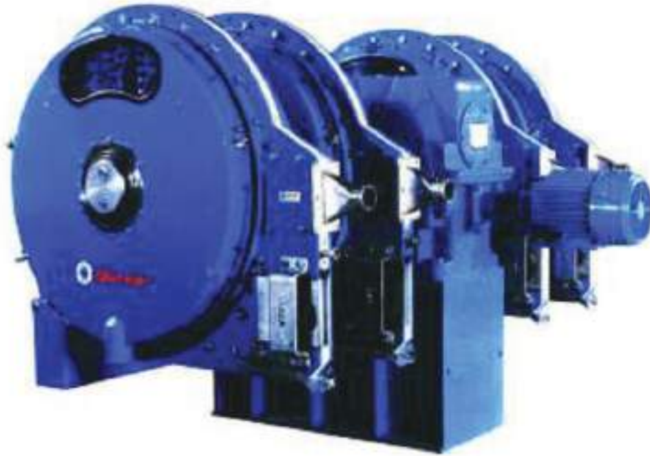
Figure 6.16 Rotary press dewatering machine (1,200φ, 4 channels)
