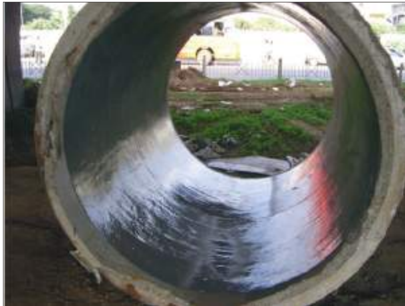
Figure 3.59 RCC Sewer pipe with protective coating
