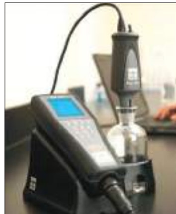
Figure 5.55 Principle of a dissolved oxygen probe
