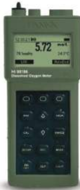
Figure 5-59 Portable BOD test instrument
